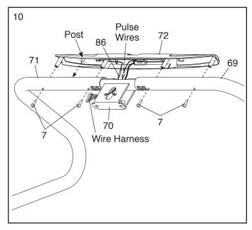
11. Hold the handrail assembly near the console assembly. Connect the wire harness extending from the handrail assembly to the wire harness extending from the console assembly. See the inset drawing in step 7. The connectors should slide together easily and snap into place. If they do not, turn one connector and try again. IF YOU DO NOT CONNECT THE CONNECTORS PROPERLY, THE CONSOLE MAY BECOME DAMAGED WHEN YOU TURN ON THE POWER.
